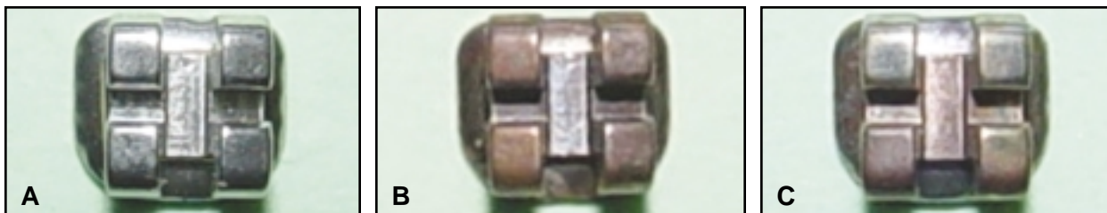
Fig. 2 A. New bracket. B. Bracket recycled with flame and microetcher. C. Bracket recycled with flame and acid bath.
